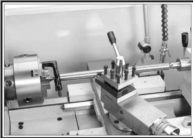
Figure 60. Example of round stock mounted between the centers.
