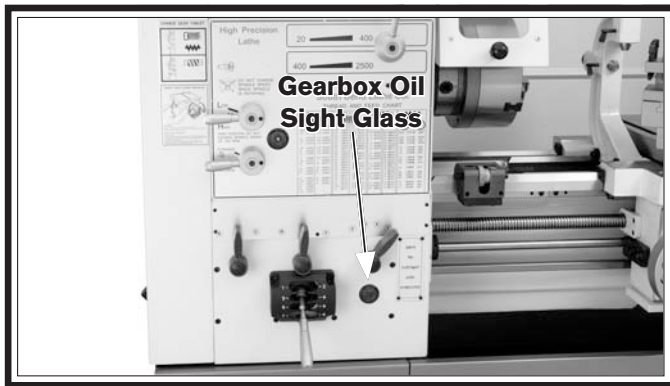
Figure 112. Gearbox sight glass location.
