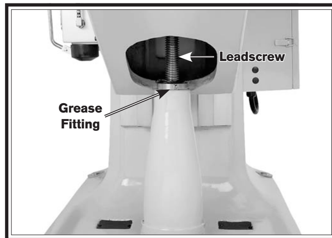
Figure 56. Table elevation leadscrew and grease fitting.
