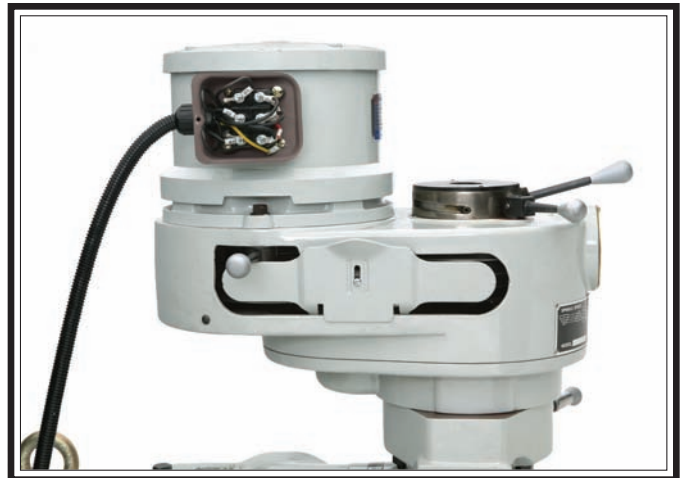
Figure 74. SB1025 Motor junction box.
