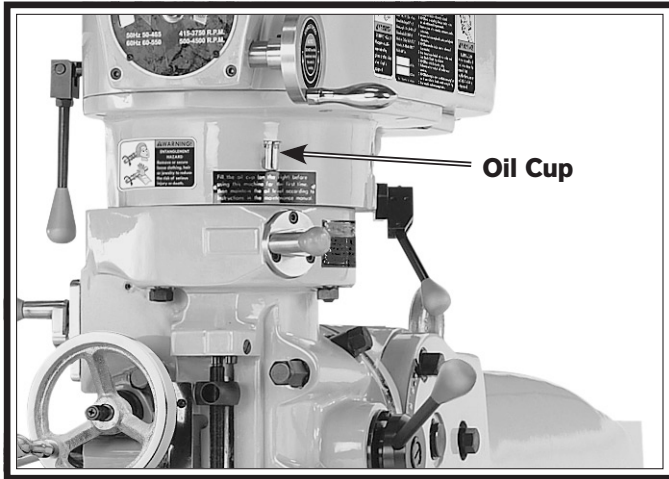
Figure 51. Speed range bearing sleeve (SB1024 only).
