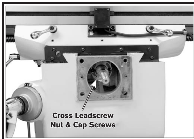
Figure 67. Cross leadscrew nut and cap screws.
