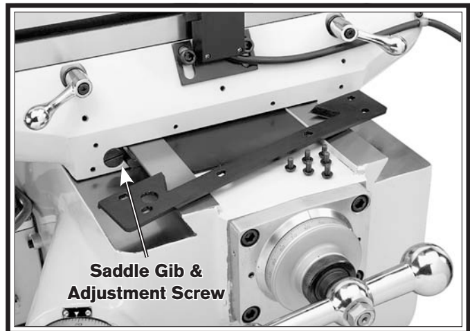
Figure 62. Saddle gib and adjustment screw.
