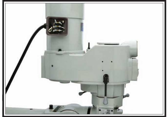
Figure 70. Motor junction box.
