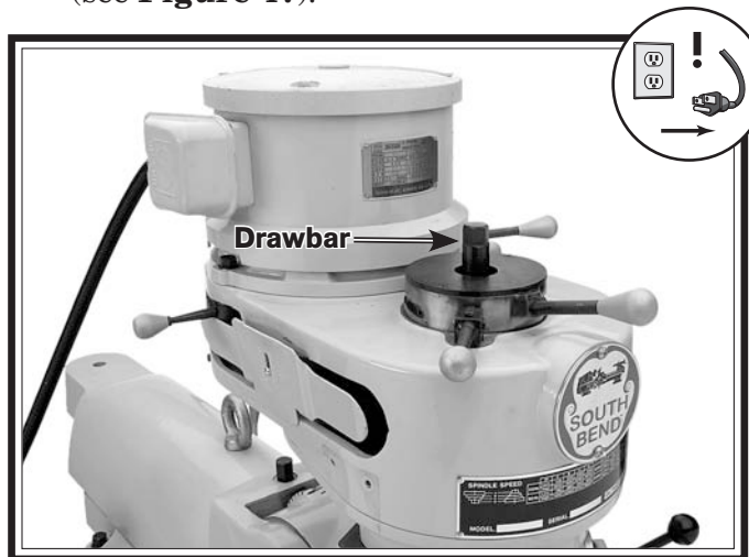
Figure 47. Drawbar loading into the spindle (Model SB1025 shown).
