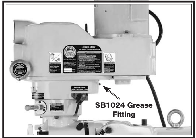
Figure 52. SB1024 headstock gearing grease fitting.
