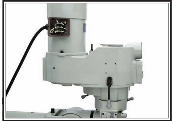
Figure 70. Motor junction box.
