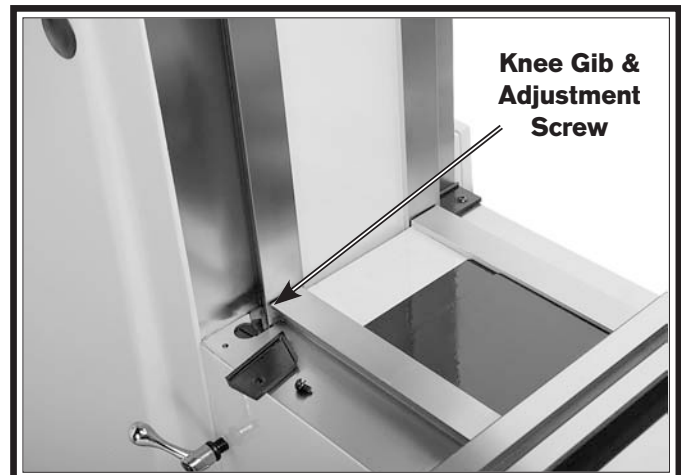
Figure 63. Knee gib and adjustment screw.
