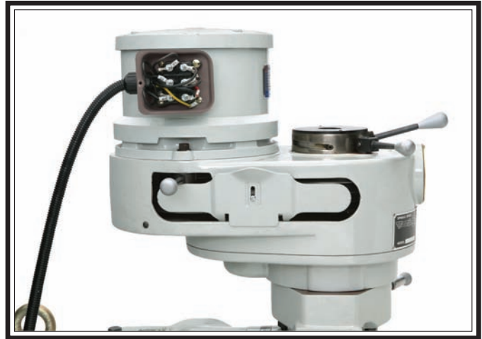
Figure 74. SB1025 Motor junction box.
