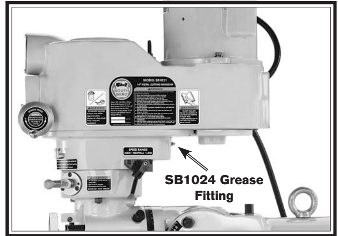
Figure 52. SB1024 headstock gearing grease fitting.
