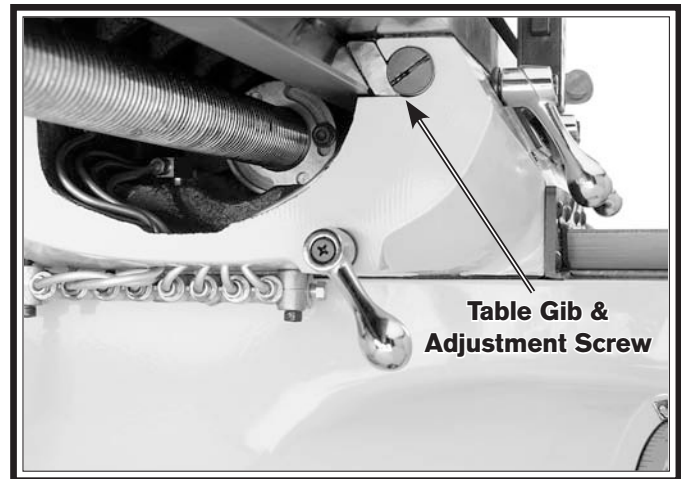
Figure 61. Table gib and adjustment screw underneath the left side of the table.
