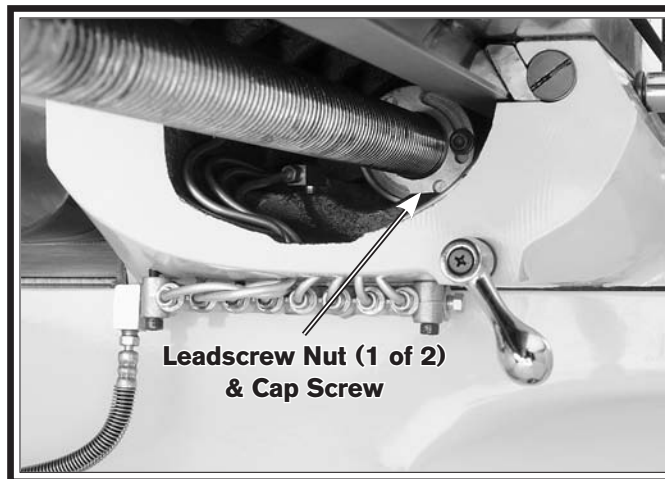
Figure 63. X-axis leadscrew nut and cap screw, as viewed from underneath the left side of the table.
