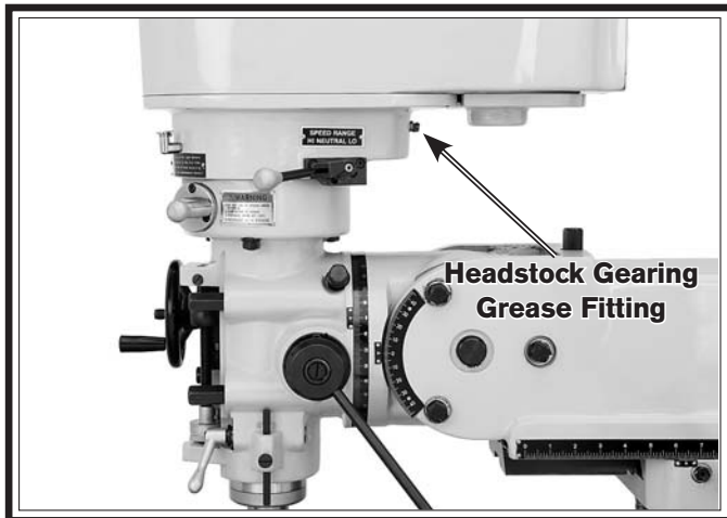
Figure 52. Headstock gearing grease fitting.
