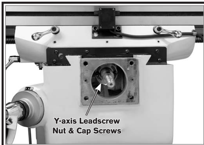
Figure 66. Y-axis leadscrew nut and cap screws.
