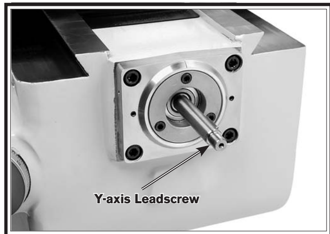
Figure 64. Ball handle, rings, and key removed from the Y-axis leadscrew.
