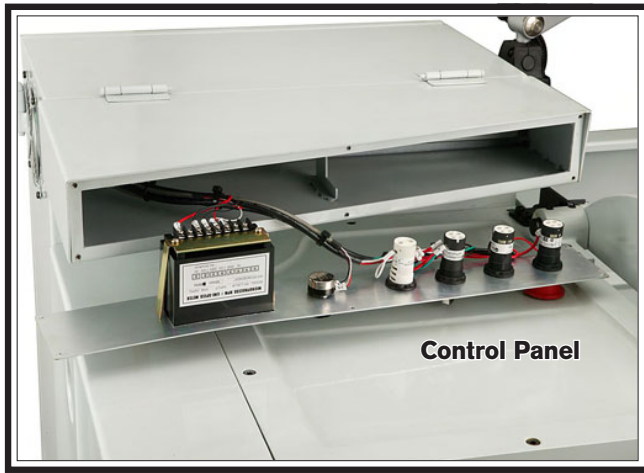
Fig. 9. Control panel location.
