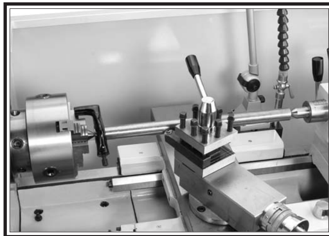
Figure 67. Example of stock mounted between the centers.
