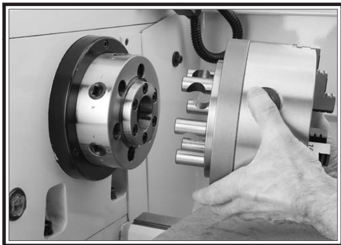
Figure 37. Example of removing a 3-jaw chuck from a spindle nose.
