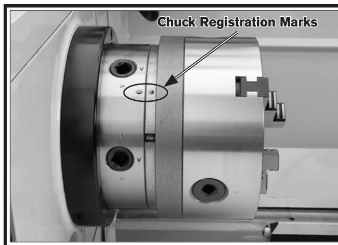
Figure 38. Chuck registration marks aligned.
