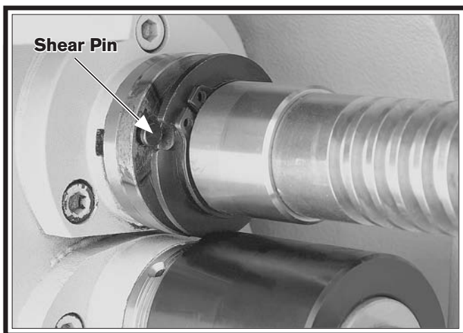
Figure 146. New shear pin installed in bore.
