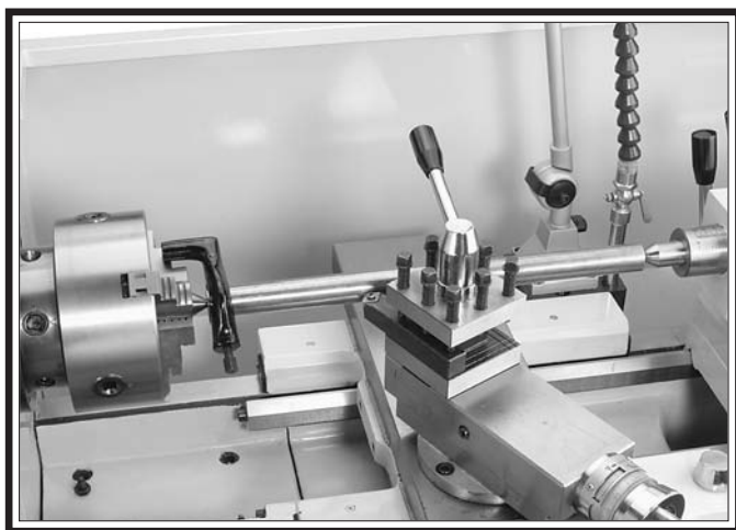
Figure 59. Example of a workpiece mounted between the centers.
